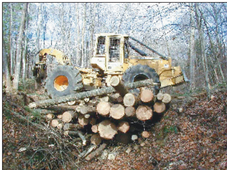
Figure 23A. Pole crossing.
